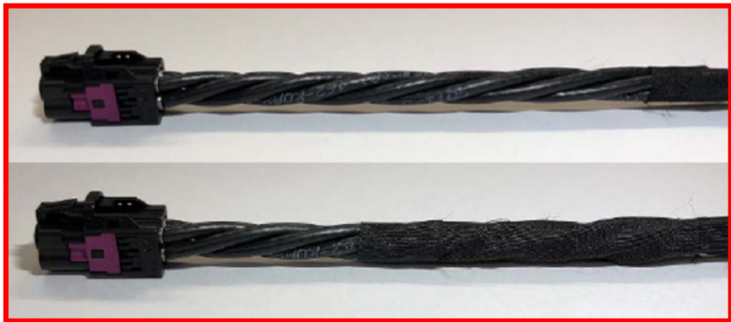
Figure 5-7 Incorrectly taped cables (example: 4-pin connector system)
