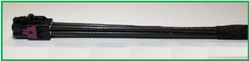
Figure 5-6 Correctly taped cable (example: 4-pin connector system)
