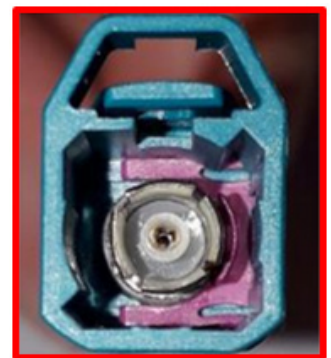
Figure 8-8 Example: Damaged connector
