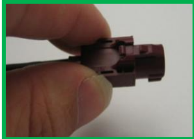
Figure 6-6 Correct handling (example: HSD)
