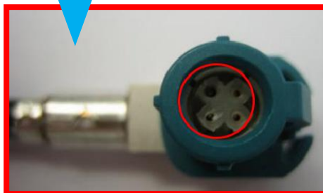
Figure 8-8 Example: HSD connector
