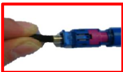
Figure 6-1 Incorrect handling (example: HSD)
