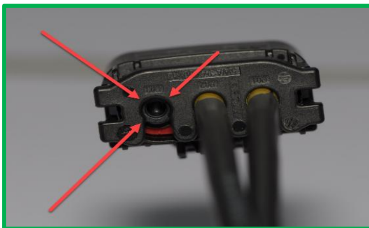
Figure 5-9 Check of blind plug (example: AMEC)
