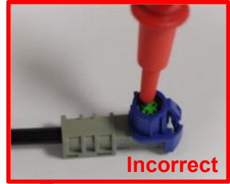
Figure 8-7 Example: HSDe connector
