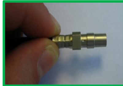
Figure 6-7 Correct handling (example: HSD)
