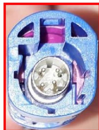
Figure 6-12 Incorrect mating (example: HSD)
