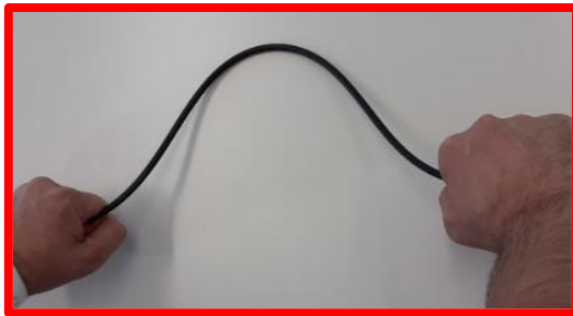
Figure 4-1 Incorrect handling (example: impulse)
