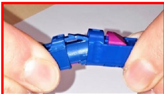
Figure 6-11 Incorrect mating (example: HSD)
