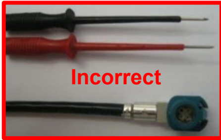
Figure 8-6 Example: HSD connector
