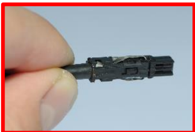
Figure 6-3 Incorrect handling (example: AMEC)
