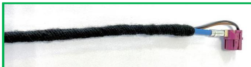
Figure 5-6 Taping of MQS stranded wires
